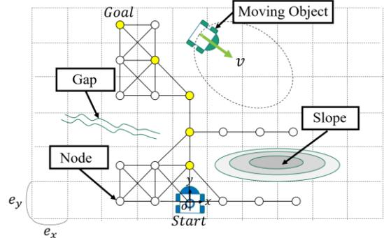
Fig.2 A graph created from the point cloud and an image of the planned path.
