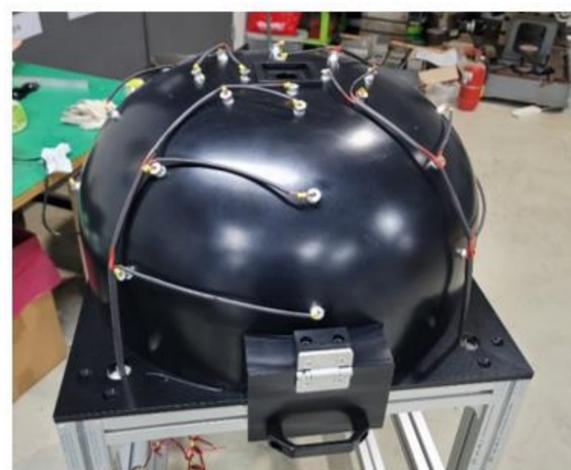
Device for measuring material reflective properties
